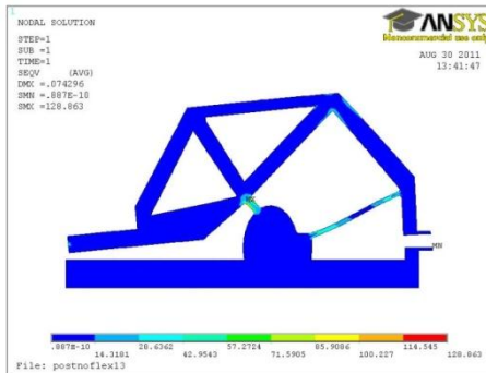
Fig.7. von-mises result obtained from FE analysis
